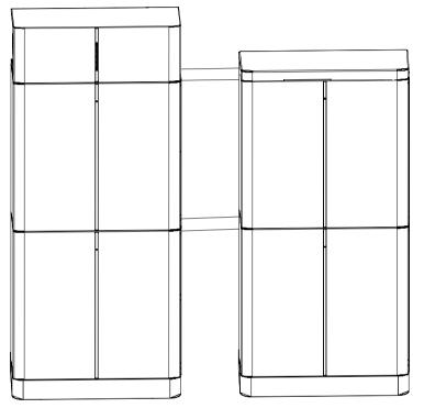
BMS + Bat x 4 Installation distance: Left: ≥300 mm Right: ≥300 mm Distance between battery columns: 200 mm ~250 mm
