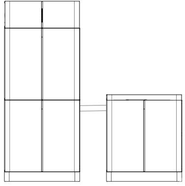
BMS + Bat x 3 Installation distance: Left: ≥300 mm Right: ≥300 mm Distance between battery columns: 200 mm ~250 mm (c)
