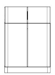
BMS + Bat x 1 Installation distance: Left: ≥300 mm Right: ≥300 mm
