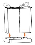
Step 3: Place the Wall Bracket, determine the position of holes, mark it with a pen, remove the Wall Bracket, and then drill the two holes (10 mm). Step 4: Place Expansion Bolts into the holes.
