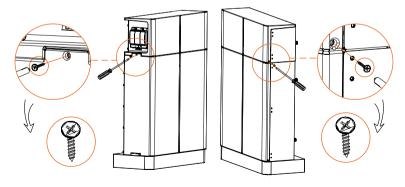
Note! Don't forget to screw both left and right sides of battery modules installed. The above steps also apply to place 2 battery modules ("b" on the page 16).
