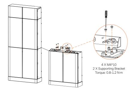
Step 2: Put the cover on the battery module. See figure below.
